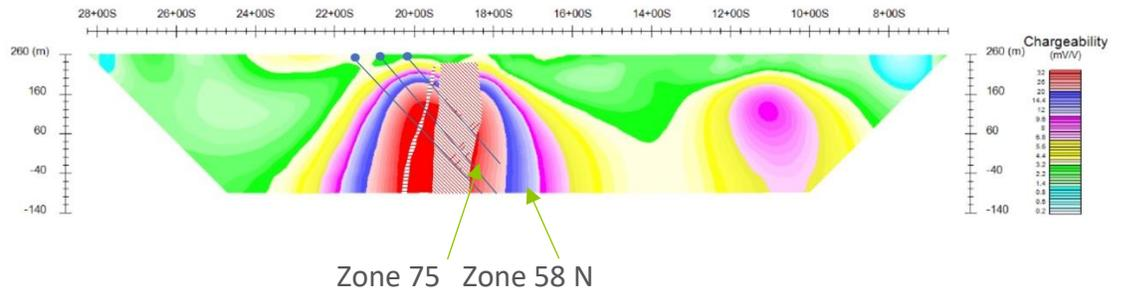
An OreVision test-survey was completed to evaluate the potential of this IP technique to discover mineralization similar to Zones 58N & 75, previously discovered by geology. The 3D inversion of the OreVision test-survey successfully delineated 2 chargeable bodies consistent with the known mineralization.
